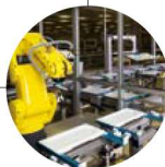
Robotic filling of bags with solution
