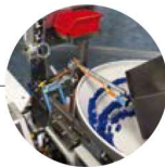
Automatic supply of hose with empty coil detection
